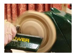
Roy's method is trial and error – use a parting tool to cut in at a very shallow angle (about 1°). The angle
