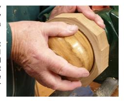
Jam chucks can be made out of any scrap piece of wood left over from a previous project, so never throw any wood away! Roy prefers to use softwood for jam chucks.
